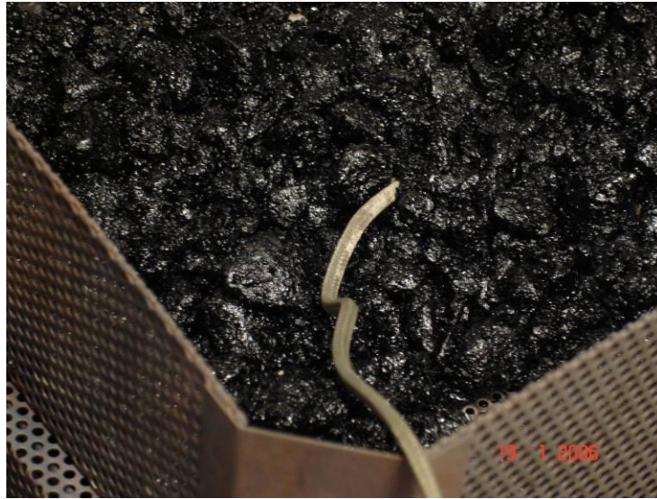
Figure 3.8. Thermocouple junction embedded in the HMA.
